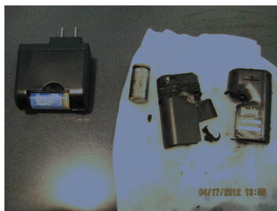
Figure 1. Photo of Mini Air Purifying Device after lithium-ion battery fire on flight from Toronto, Canada, to Minneapolis/Saint Paul, Minnesota, 17 April 2012.
